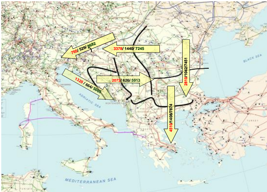
Figure 4. Bulk power flows in Vision 4
