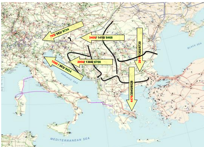
Figure 1. Bulk power flows in Vision 2
