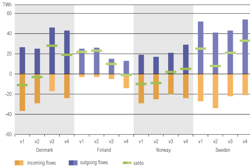
Figure 96 Annual inter-area flows in Nordic countries for different visions. Positive value is corresponding to total outgoing flows and negative value to total income flows.
