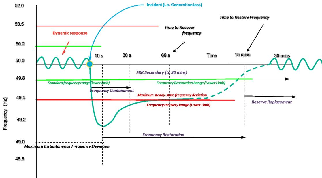
5. The above diagram shows an illustration of frequency behaviour that obeys the rules of SOGL and GB electricity codes.
