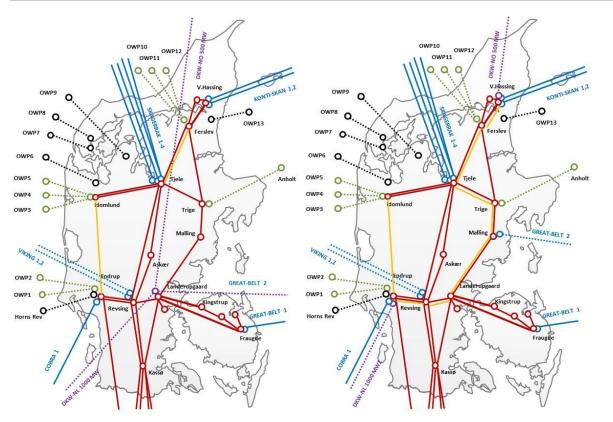
Figure 7.24 - (Left) – Multi-terminal HVDC connection and (Right) – Point-to-point HVDC connectors to Denmark-West. Colour legend: Blue – HVDC connectors prior to Common Planning Studies; Red – the Danish 400 kV transmission system prior to Common Planning Studies; Yellow = 400 kV grid reinforcements needed; Violet = potential HVDC connectors to Denmark-West.
