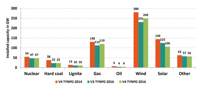
Figure 4.11: Installed capacity in GW in the North Sea Region
