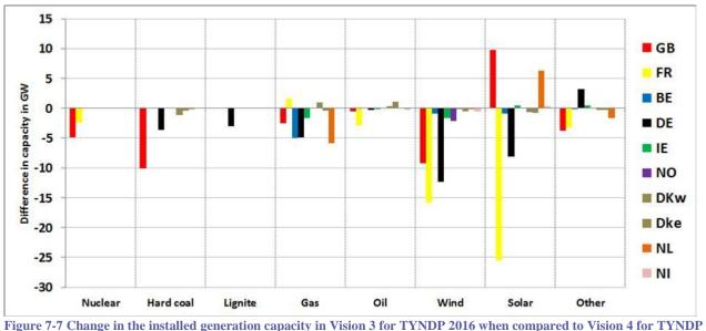
Figure 7-7 Change in the installed generation capacity in Vision 3 for TYNDP 2016 when compared to Vision 4 for TYNDP 2014.
