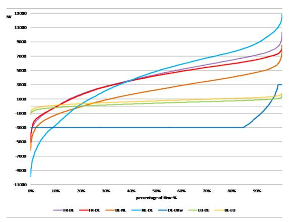
Figure 4.7: Power flow duration curves on the AC borders within the Continent<sup>1</sup>
