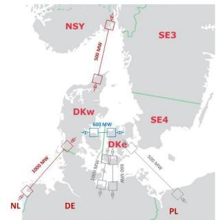
Figure 7-21 – HVDC potential projects to Denmark-West, shown as point-to-point connectors, which can be relevant for merging into a multi-terminal HVDC system. Marking: blue –TYNDP-2014 projects, red – potential new projects, grey – connectors to Denmark-East which are analysed within Regional Group Baltic Sea.
