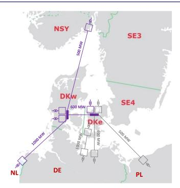
Figure 7-23 – HVDC potential projects merged into a multi-terminal HVDC system with a HVDC hub. Marking: violet – a multi-terminal HVDC system, red – a point-to-point connector, grey – candidate projects in Denmark-East (analysed in Regional Group Baltic Sea).
