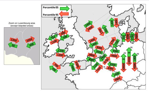
Figure 4.6: Bulk power flows – 5<sup>th</sup> (green) and 95<sup>th</sup> (red) percentiles resulting from the increased transfer capacities
