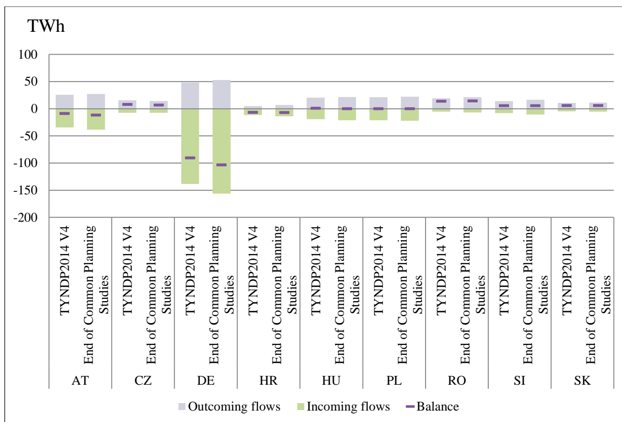
Figure 4-6 Country power balance TYNDP 2014 in comparison to the end of Common Planning Studies
