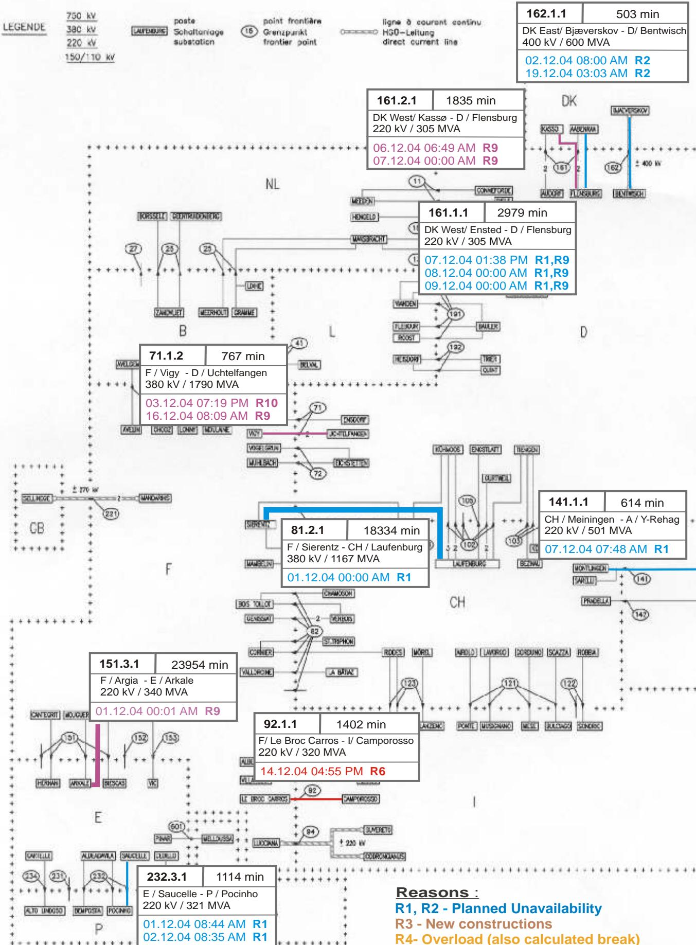
**Reasons :****R1, R2 - Planned Unavailability****R3 - New constructions****R4 - Overload (also calculated break)****R4, R5, R6 - Failed transmission network****R7, R8 - External impacts****R9, R10- Other reasons**
