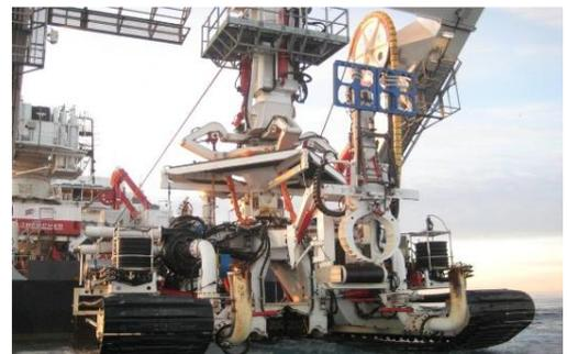
*Trencher used by Eirgrid for burying the cable of the East-West Interconnector*
