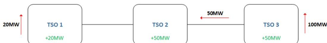
Figure 3: Example Interconnection Controllability: results of unconstrained run
