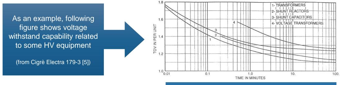
Withstand TOV characteristics for power equipment
